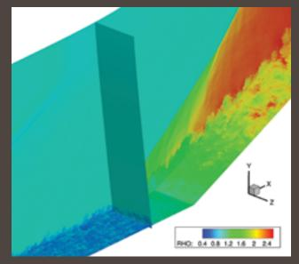
A close up of the separated flow over a ramp at Mach 2.25 shows the complex turbulent flow near the bottom wall and unsteady shocks farther away. From work carried out by Kevin Porter (MS '17) under Poggie s DoE INCITE Award.
