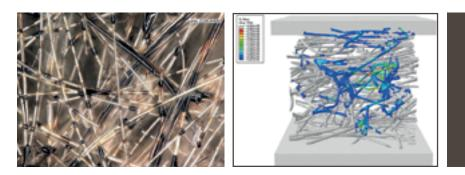
In an example of how simulation based engineering can assist manufacturers, Purdue demonstrated to Knauf Insulation how mechanical loads are transmitted in porous glass fiber materials. PHOTOS: COLLEGE OF ENGINEERING
