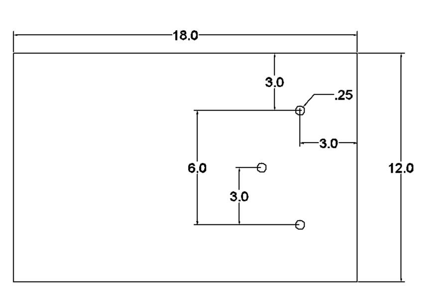
Fig 2. Shows the plate designed to be welded onto the bottom of the chassis dyno and secured down with concrete fasteners.
