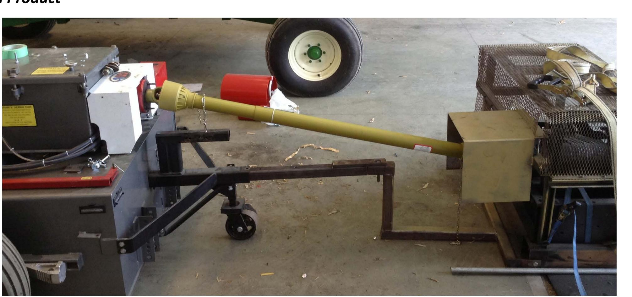
Fig 3. Shows the finished "Dual Dyno" system mounted to the floor and ready for initial testing.
