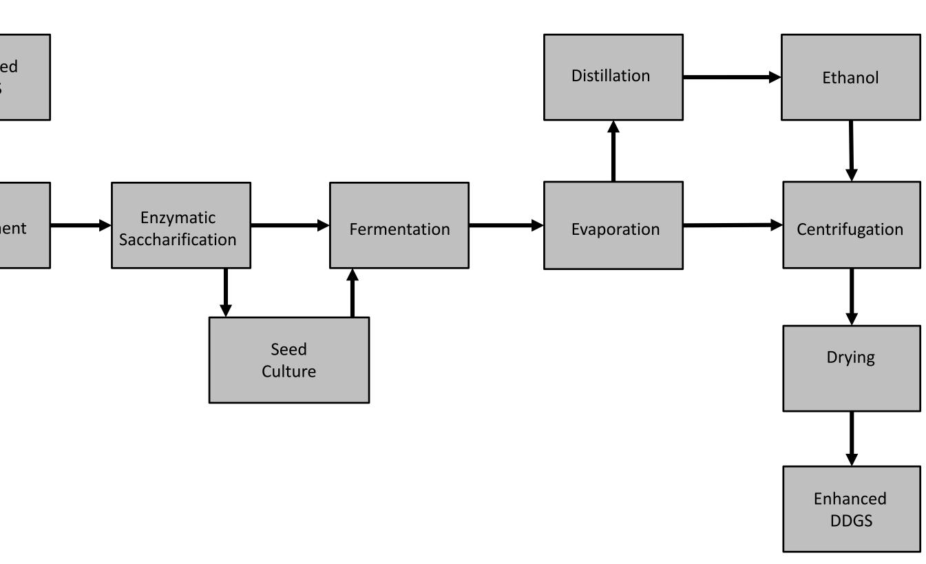
Pretreatment Before a biomaterial can be converted to any form of simple sugar, it needs to be pretreated. We will pretreat the DDGS by adding liquid hot water to it while controlling the PH of the solution. The heat of the liquid will disrupt the cellulose chain, solubilizing it and preparing it for the hydrolysis process so a more efficient reaction occurs
