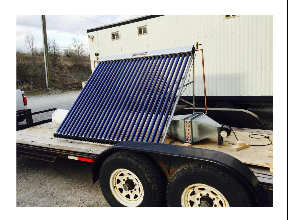
Figure 3: Front view of the completed prototype.
