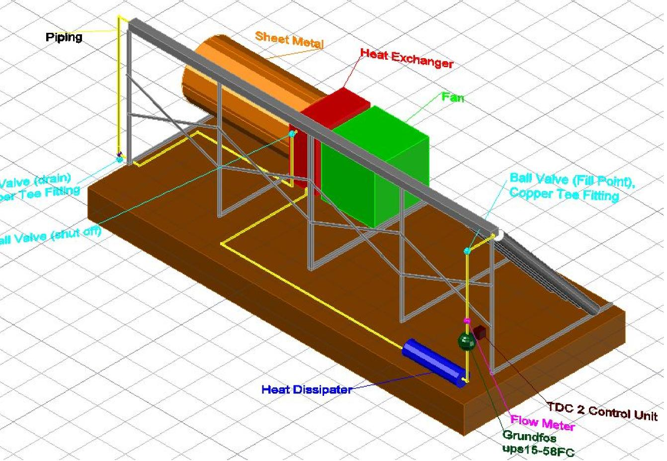
**Figure 1:** The fourth version of our design produced in AutoCAD.
