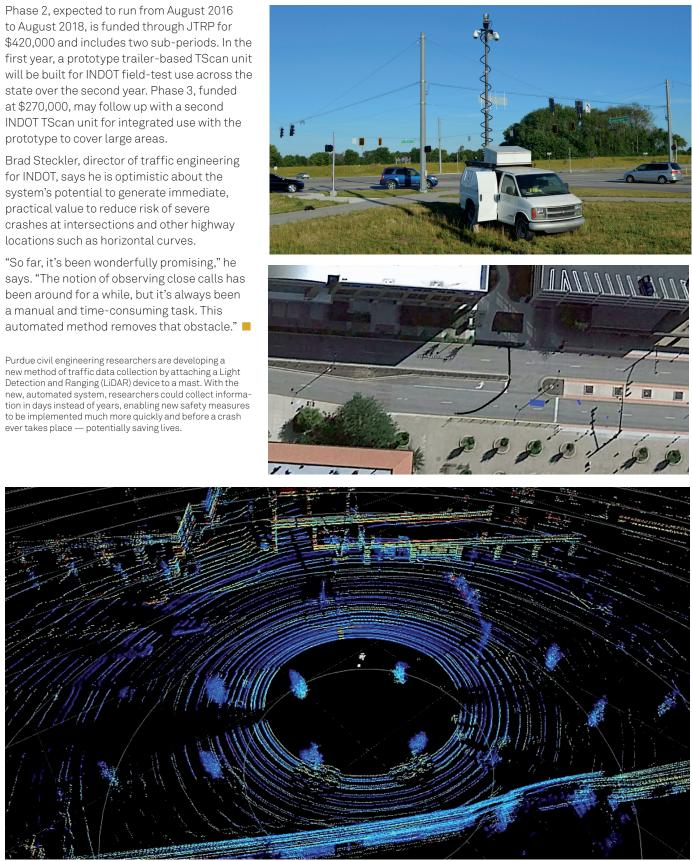
Purdue's School of Mechanical Engineering is assisting in the study. Through a software program ME created, the raw data collected from the LiDAR technology is translated from countless dots on a black screen to a fully mapped traffic area, complete with data points that detail the speed of objects and pedestrians and their proximities to each other
