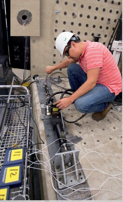
PhD candidate Christian Silva tests a magneto-rheological damping system, which provides variable damping under earthquake loading. The work is part of Professor Shirley Dyke's Intelligent Infrastructure Systems Lab in Purdue's Robert L. and Terry L. Bowen Laboratory for Large-Scale Civil Engineering Research. Photo: Mark Simons, Purdue
