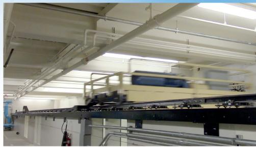
The towing tank's carriage runs on rails and can move as fast as five meters per second. The carriage is used to haul objects through the water-filled tank (below) to quantify flow patterns and hydrodynamic forces.
