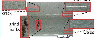
(b) Scratches, grind marks, and welds in background.
