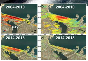
Perissin's team developed a multisensor cumulative deformation map for the dam based on satellite data. (Image source: Daniele Perissin, Nature.)
