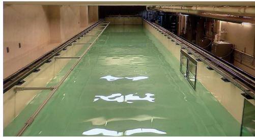
The towing tank, a 150-foot-long, 11-foot-wide and five-foot-deep water basin, will be used for coastal engineering and fluid dynamics research in the Burke Lab.
