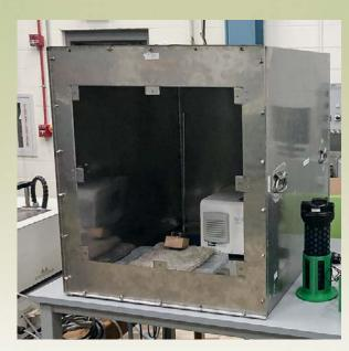
Brian Magnuson, an undergraduate student researcher, helped design and build a full-scale environmental chamber to conduct dust transfer experiments.
