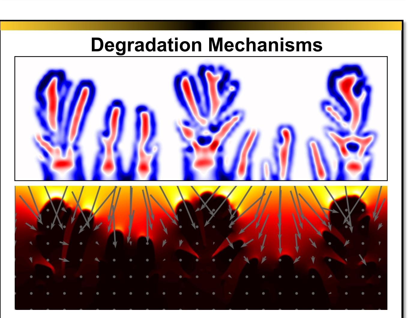
Lithium dendrites (see images above) are electrodeposits that nucleate and grow on battery anodes during recharge (see image in Introduction). Unchecked dendrite growth leads to short circuits and causes catastrophic battery failures. In this project, we develop a unified theoretical framework that delineates growth mechanisms (e.g., tip- and base-controlled growth), as a stepping stone to identify battery fabrication strategies that enable safer, improved devices.
